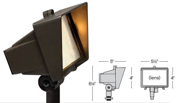
1521 BZ FLOOD LIGHT WITH FROSTED LENS 5 1/2" W, 4" H SHROUD 5" W, 6 1/4" H
