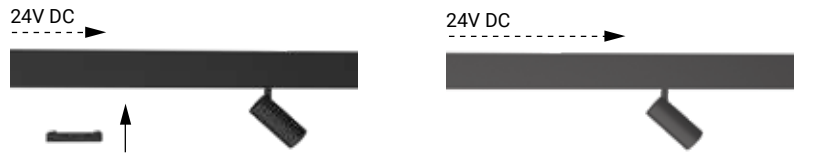
Using circuit joint (36362-01) to connect between tracks
